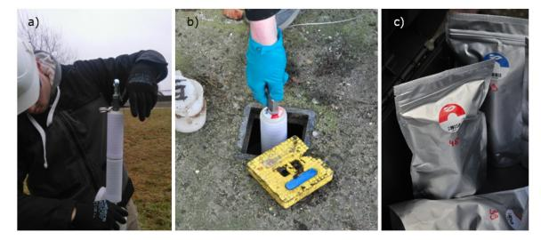
Figure 3: iFLUX application in the field a) iFLUX sampler with 2 cartridges, b) VOC cartridge on sampler that slides in monitoring well, c) iFLUX cartridges in their packaging bags.
